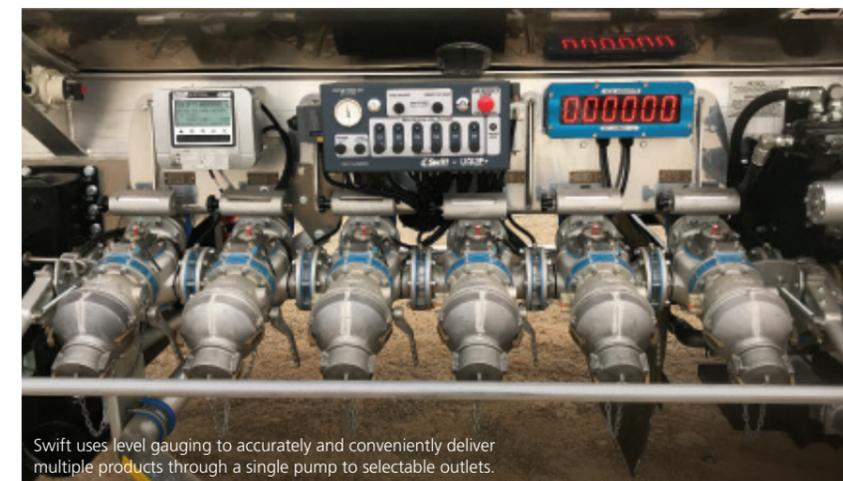
Swift uses level gauging to accurately and conveniently deliver multiple products through a single pump to selectable outlets.
