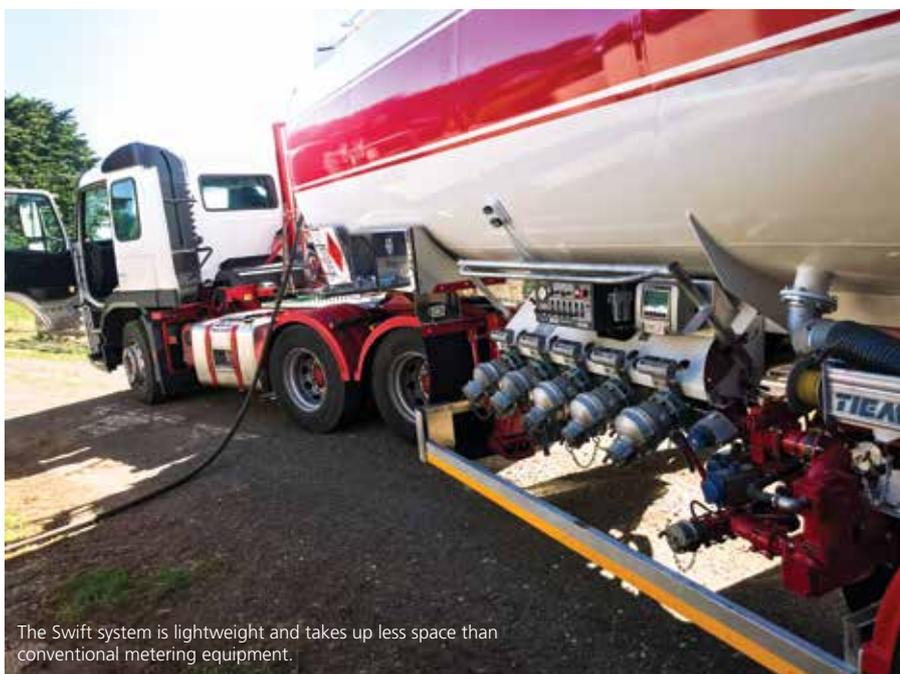
The Swift system is lightweight and takes up less space than conventional metering equipment.
